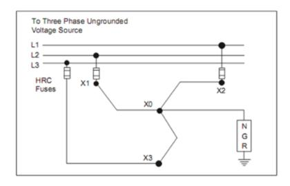
Zigzag. Since these three currents are all equal and in time phase with each other (zero sequence), and because of the special Zigzag winding connections, they see a very low impedance. This allows the ground fault current to flow back into the system. It can be seen that the ground fault current is only limited by the resistance of the ground fault, the NGR, and the small reactance of the Zigzag.
